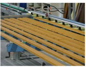
Vacuum painting is the latest technology for painting of the profiled wood. This method is of higher quality and quicker than other conventional methods. Painting is performed in a vacuum chamber where paint is spread. Due to this technology all surfaces of the wood are evenly covered with paint. Vacuum painting method ensures wood surface resistance to climate effects and protects it from the mould spores.
